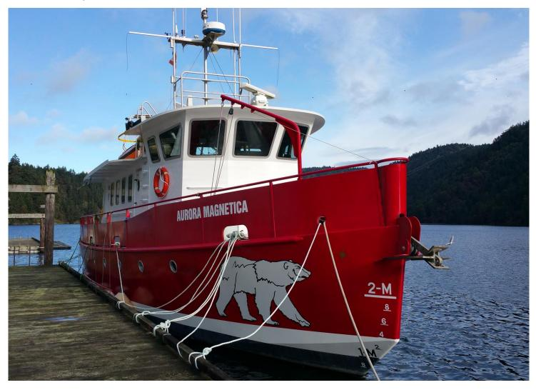
The ship was constructed with an aluminum hull capable of withstanding the forces of ice. She has a very shallow draft and is designed to be beached on her flat bottom hull in low tides. Since 2004, the Aurora Magnetica has served as a platform for research activity, film crews, as well as personal travelers primarily throughout the Canadian arctic in Greenland.
